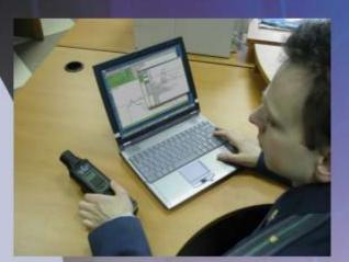
The radionuclide spectra libraries being used for identification can be selected and the instrument can be applied for resolving specific tasks
